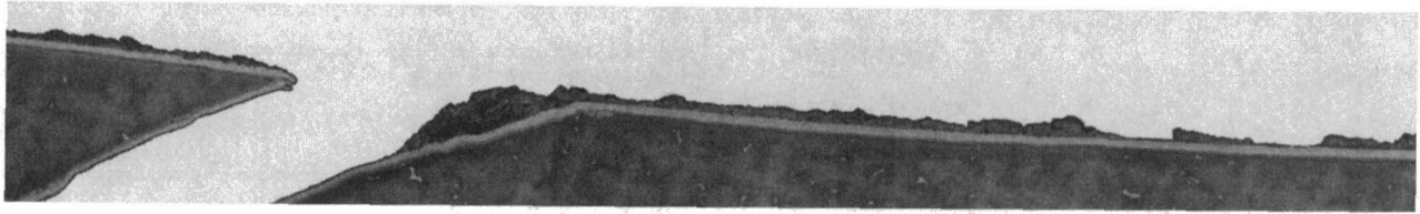
Fig. 2 Micrograph showing roughness caused by deposits of foreign materials along the surface and in a film cooling hole
